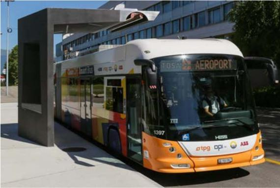
Figure 10.4 Mobile Pantograph
