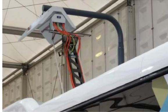
While there are less well-known pantograph systems, with the agreement recently concluded in Europe, they are unlikely to progress past the prototype stage. It should, however, be noted a wide variety of presentations of these two types of pantographs exist; and many of them are aesthetically appealing, enabling City planners to integrate them with other street furniture.
