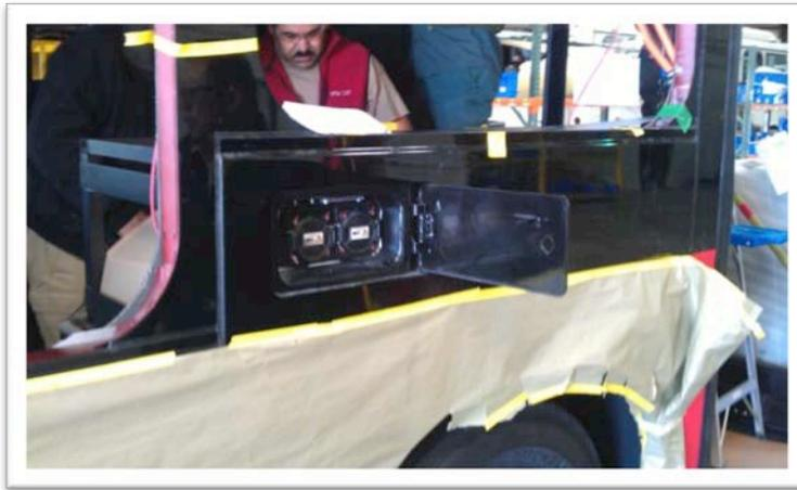
The NFI connector is heavy and normally, an operating garage would be supplied with a connector support that was not available for the ETS test program.
