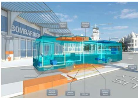
Figure 10.6 Mobile Induction Plate
