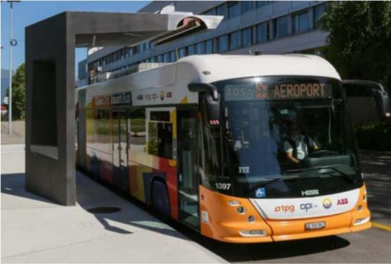
Figure 10.4 Mobile Pantograph
